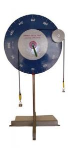
Apparatus consists of a metallic pulley of 30 cm diameter with two grooves, one for rope and the other for belt. At back side of the pulley, a circular wooden disc is provided with graduation at 10<sup>0</sup> intervals. A rotating pulley is fixed at the circumference of the scale. Apparatus is supplied complete with one belt and rope. The apparatus is mounted on a heavy vertical stand.
